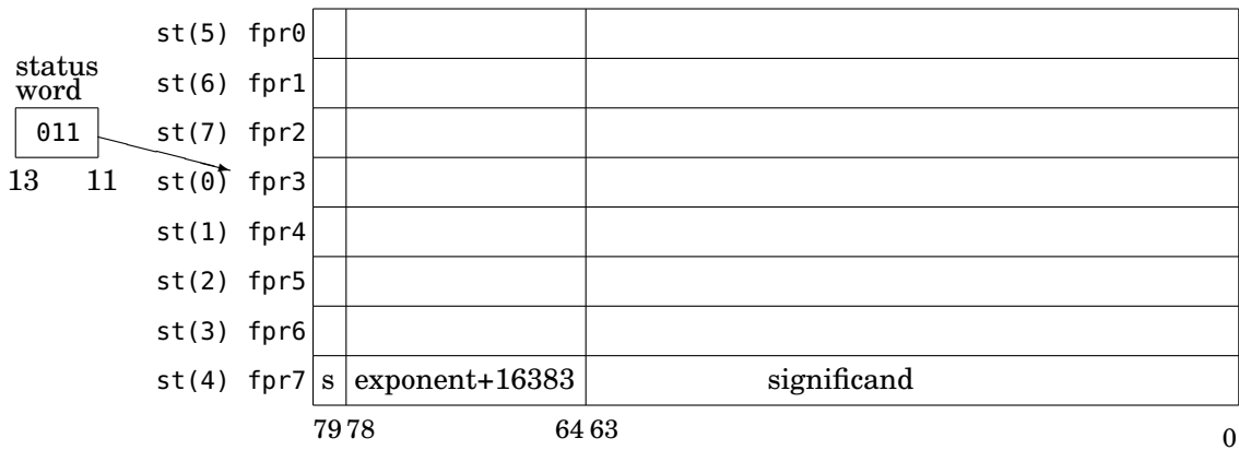
Figure 14.2: x87 floating point register stack. The fpr i represent the absolute locations. The st( j ) are the stack names, which are used by the instructions. In this example the top of the stack is at fpr3 , as shown in bits 13 – 11 of the x87 status register.
